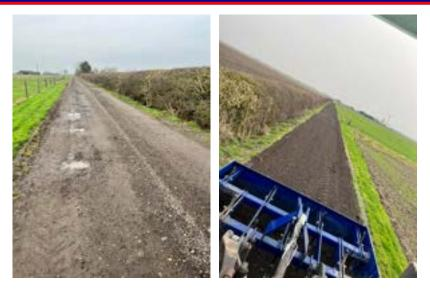
The Oxdale heavy duty grader is ideal for use on farm tracks and drives. Durable tines easily break up the ground surface. Debris is dragged in the box to where the ground is lower where it is then deposited. Rear blades level and grade the ground surface. Available in 6ft, 8ft and 10ft models.
