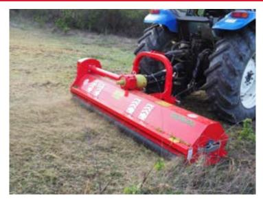
The Levante is suitable for heavy duty use on hard and uncultivated soils. The honeycomb structure and high thickness allows you to cut bushes and pruning of big diameter shrubs getting excellent results. The Levante flail mower is suitable for 80-120hp tractors with CAT2 3-point linkage. The Levante mower is supplied with a universal CAT6 PTO shaft, hydraulic side shift.
