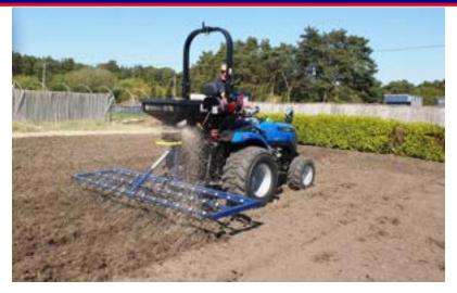
The Oxdale fixed weeder has revolutionised grass harrowing in recent years. The weeder is available in multiple sizes perfect for small and compact tractors. The Oxdale weeder has aggressive spring tines meaning that a better finish can be achieved faster and at a lower cost.
