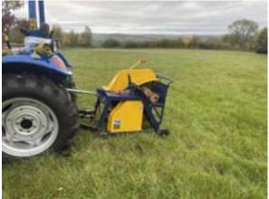
The Oxdale PTO saw bench is perfect if you have a low to medium HP tractor . The PTO saw bench allows the user to cut logs up to 12" in diameter. The swinging cradle allows the cutting process to a be quick, safe and efficient.
