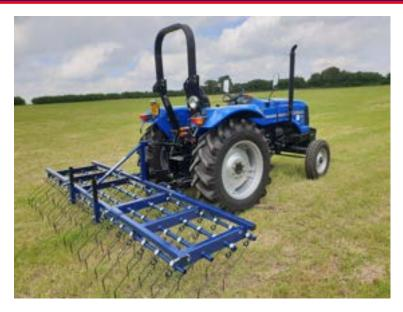
The Oxdale folding 12ft weeder has revolutionised grass harrowing in recent years. Larger working widths, more adjustment and aggressive spring tines mean that a better finish can be achieved faster and at a lower cost.
