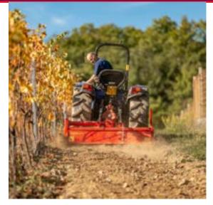
The Eagle rotary tiller combines style, functionality and power to break up the ground. Easy to use and a powerful piece of machinery used to carry out all the functions related in various working environments in all types of ground whatever its composition (sandy soil, medium mixture or clay).
