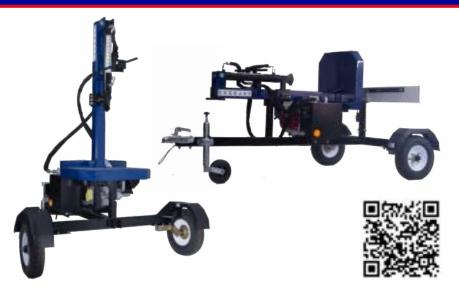
The RT400 is a fully road legal towable log splitter. The RT400 is powered by a 6.5hp Honda GX200 engine which is teamed with the dual speed hydraulic pump, giving you an exceptionally strong 10 ton splitting force.
