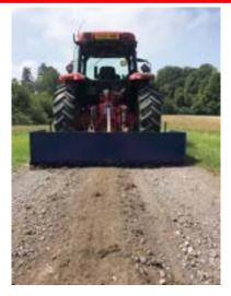
The medium duty grader was developed for users with medium HP tractors. The medium duty grader will stand higher than the standard with 10mm thick steel sides. The back of the machine is made from one piece of sheet metal with added strengthening.
