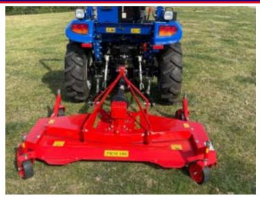
The Del Morino Finishing Mower with belt drive are suitable for tractors which are 12-70hp with CAT1 three-point linkage. The cast iron gearbox with free wheel produces 540rpm. The mower is supplied with a universal PTO shaft CAT2.
