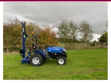
The Oxdale Post knocker is suitable for use with all tractors. The post knocker has 60kg (max) weight block which can be reduced by removing leaves. A bolt-on, side mount bracket is also available should you wish to use the post knocker with a loader or digger.
