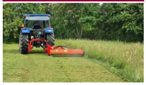
The Levante Super Flail Mower has all the characteristics of the standard Levante with added manoeuvrability. This machine is suitable for heavy duty use on hard and uncultivated soils for the professional user. It's honeycomb structure with high thickness cover and walls (side walls 10mm) allows the user to cut grasses, bushes, stubble, reeds and even pruning of big diameter saplings – getting good results. For
