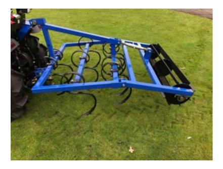
Spring Tines are a necessity for operators in farming, smallholding, landscape development or estate management. Spring Tine Cultivators are a productive tractor attachment, they are available in a range of widths 4-foot, 6 foot and 8 foot.
