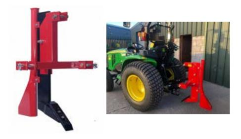
The Oxdale ripper and pipe layer is perfect for laying pipes or cabling around paddocks or fields, for pipes up to 4.5cm. The glides smoothly through a variety of ground types. Ripper adjustable height settings 18-24 inches.
