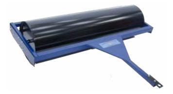
The paddock roller is water ballasted which makes it ideal for grassland work. The Oxdale land roller is fitted with a pin or 50mm standard ball hitch towing point and can be towed by tractor, ATV or 4×4.
