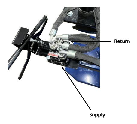
The flow and return pipes have been fitted with male ½" quick release couplings. The supply pipe is connected to the control valve and is marked "P." The free flowing return is marked with a "T." Connecting these pipes the wrong way round can damage the control valve.
