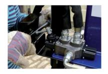
The handle will return itself to the neutral position when not lifted or lowered. In this position, here will be no movement of the wedge.
