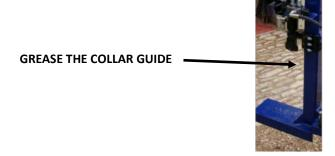
Any grease can be used to carry out this action. The grease will allow the ram to move smoothly up and down, making splitting much easier.
