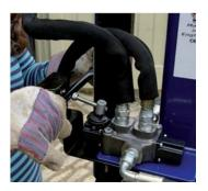
With both hands grasp the safety levers and squeeze the handle, lift to lower the wedge.
