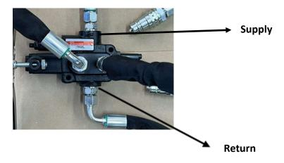
The flow and return pipes have been fitted with male ½" quick release couplings. The supply pipe is connected to the control valve and is marked "P." The free-flowing return is marked with a "T." Connecting these pipes the wrong way round can damage the control valve.
