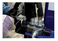
The handle will return itself to the neutral position when not lifted or lowered. In this position, there will be no movement of the wedge.
