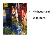
Connecting hydraulic hoses to the tractor with the engine switched off:
